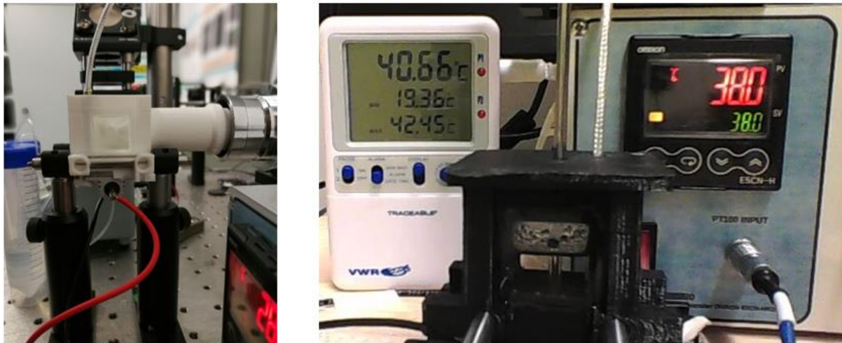
Figure 4. Arrangement for temperature stability tests: (left) Detail of the temperature sensor and the heating pad attached to the chamber and (right) Detail of the temperature measuring points, one on the corner and another in the centre of the chamber.
